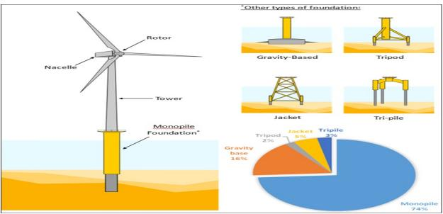
Figure 1: Offshore Wind Turbine Foundation types
