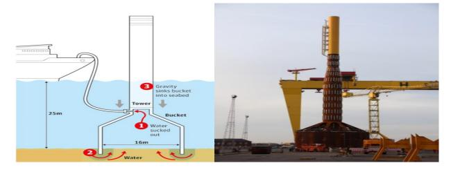
Figure 2a: Schematic Diagram of the Mono Bucket
