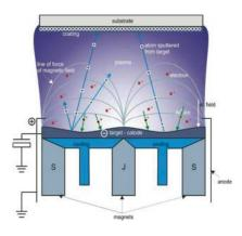
Figure 4: Sputtering Process<sup>17</sup>
